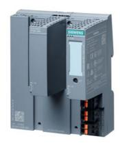
SCALANCE XF204-2BA managed IE switch, 4 x 10/100 Mbit/s, IEC 62443-4-2 certified; 2 x BusAdapter interface, error signaling contact, set pushbutton, redundant 24 V DC power supply, PROFINET device, extended temperature range -40 °C...+70 °C, conformal coating, with electr. manual on DVD, C-PLUG optional, supplied without BusAdapter
