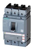
circuit breaker 3VA5 UL Frame 250 breaking capacity class C 100 kA @ 480 V 3-pole, line protection TM230, FTAM, In=90 A overload protection Ir=90 A permanently set short-circuit protection Ii=5...10 x In UL489 SB (naval), 50 degrees Celsius cable connection on two sides
