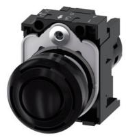
acoustic signal device, compact, 22 mm, round, plastic, black, Continuous tone 2.4 kHz, IP40, Sound pressure min. 80 dB/10 cm, with holder, Operating voltage 24 V AC/DC, screw terminal, Z=50-unit packaging
