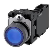
Illuminated pushbutton, 22 mm, round, plastic with metal front ring, blue, pushbutton, flat, momentary contact type, with holder, 1 NO+1 NC, LED module with integrated LED 24 V AC/DC, screw terminal, with laser labeling, inscription or symbol Customer-specific selection with SIRIUS ACT configurator (CIN)
