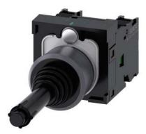
Coordinate switch, 22 mm, round, plastic with metal front ring, black, 2 switch positions, horizontal latching, with mechanical interlocking, in O position, with holder, 1 NO, 1 NO, screw terminal, with laser labeling, upper case and lower case, always upper case at beginning of line
