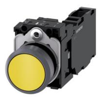
Pushbutton, 22 mm, round, plastic with metal front ring, yellow, pushbutton, flat, momentary contact type, with holder, 1 NO+1 NC, screw terminal, with laser labeling, inscription or symbol Customer-specific selection with SIRIUS ACT configurator (CIN)
