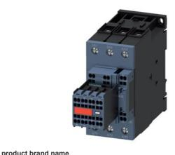
power contactor, AC-3e/AC-3, 41 A, 18.5 kW / 400 V, 3-pole, 20-33 V AC/DC, 50/60 Hz, with integrated varistor, auxiliary contacts: 2 NO + 2 NC, main circuit: screw terminal, control and auxiliary circuit: spring-loaded terminal, size: S2, captive auxiliary switch
