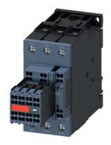
power contactor, AC-3e/AC-3, 41 A, 18.5 kW / 400 V, 3-pole, 110 V AC, 50 Hz / 120 V, 60 Hz, auxiliary contacts: 2 NO + 2 NC, main circuit: screw terminal, control and auxiliary circuit: spring-loaded terminal, size: S2, captive auxiliary switch
