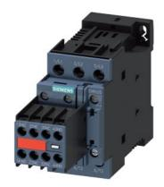
power contactor, AC-3e/AC-3, 32 A, 15 kW / 400 V, 3-pole, 24 V DC, with plugged-in varistor, auxiliary contacts: 2 NO + 2 NC, screw terminal, size: S0, captive auxiliary switch
