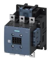
power contactor, AC-3e/AC-3 265 A, 132 kW / 400 V Uc: 24 V DC x (0.7-1.25) PLC input 24-110 V DC 3-pole, auxiliary contacts 2 NO + 2 NC drive: electronic main circuit: busbar control and auxiliary circuit: spring-loaded terminal extended rated condition railroad IEC 60077
