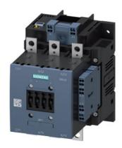
power contactor, AC-3e/AC-3 150 A, 75 kW / 400 V Uc: 24 V DC x (0.7-1.25) PLC input 24-110 V DC 3-pole, auxiliary contacts 2 NO + 2 NC drive: electronic main circuit: busbar control and auxiliary circuit: spring-loaded terminal extended rated condition railroad IEC 60077
