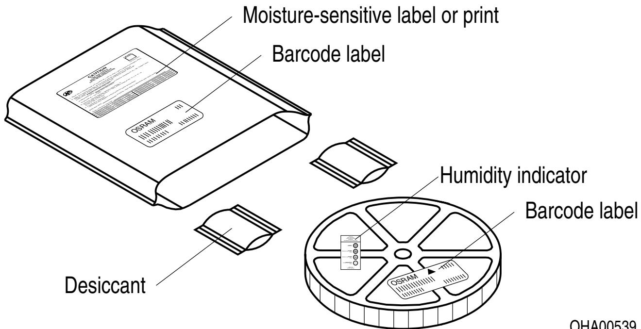
Moisture-sensitive product is packed in a dry bag containing desiccant and a humidity card according JEDEC-STD-033.
