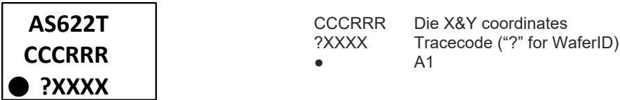
Figure 16: WLCSP package marking/code for AS6221T
