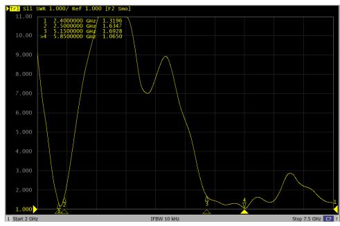
The VSWR of the antenna measured from 2 - 7.5 GHz.
