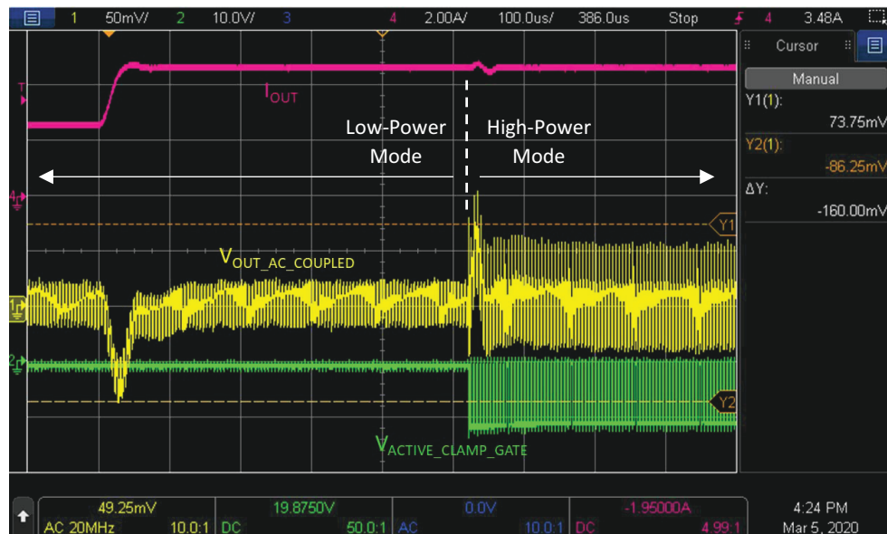
Figure 18. Low-Power Mode to High-Power Mode Transition ( I_{\text{OUT}} Changes from 2.6 A to 4.7 A)
