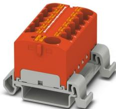
Distribution block, nom. voltage: 800 V, nominal current: 32 A, number of connections: 13, connection method: Push-in connection, Rated cross section: 4 mm<sup>2</sup>, Load contact, cross section: 0.2 mm<sup>2</sup> - 6 mm<sup>2</sup>, Push-in connection, Line contact, Rated cross section: 10 mm<sup>2</sup>, cross section: 0.5 mm<sup>2</sup> - 10 mm<sup>2</sup>, mounting type: NS 35/7,5, NS 35/15, color: red
