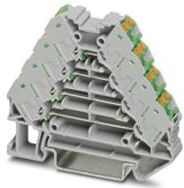
Marshalling panel, nom. voltage: 250 V, nominal current: 10 A, connection method: Push-in connection, 1st, 2nd, 3rd and 4th level, Rated cross section: 1.5 mm<sup>2</sup>, cross section: 0.14 mm<sup>2</sup> - 2.5 mm<sup>2</sup>, mounting: NS 35/7,5, NS 35/15, color: gray, color of connection elements: green
