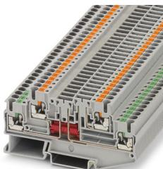
Disconnect terminal block, Current and voltage are determined by the plug used., nom. voltage: 400 V, Thermal continuous current  $I_{th}$ : 16 A, 1st and 2nd level, connection method: Push-in connection, Rated cross section:  $2.5 \text{ mm}^2$ , cross section:  $0.14 \text{ mm}^2$  -  $4 \text{ mm}^2$ , mounting: NS 35/7,5, NS 35/15, color: gray
