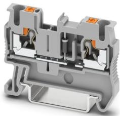
Component terminal block, The max. current is determined by the diode. Installed: Diode 1N4007, reverse voltage: 1300 V, maximum continuous current: 0.5 A., with integrated 1N4007 diode, nominal current: 0.5 A, connection method: Push-in connection, Rated cross section: 2.5 mm<sup>2</sup>, cross section: 0.14 mm<sup>2</sup> - 4 mm<sup>2</sup>, mounting: NS 35/7,5, NS 35/15, color: gray
