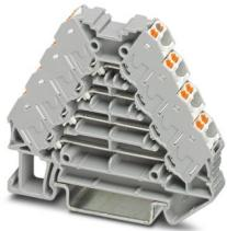
Marshalling panel, nom. voltage: 250 V, nominal current: 10 A, connection method: Push-in connection, 1st, 2nd, 3rd and 4th level, Rated cross section: 1.5 mm<sup>2</sup>, cross section: 0.14 mm<sup>2</sup> - 2.5 mm<sup>2</sup>, mounting: NS 35/7,5, NS 35/15, color: gray
