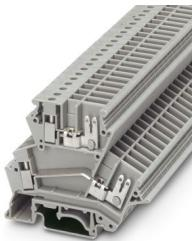
Feed-through terminal block, nom. voltage: 400 V, nominal current: 20 A, 1st and 2nd level connection left, connection method: Screw connection, Rated cross section: 4 mm<sup>2</sup>, cross section: 0.2 mm<sup>2</sup> - 4 mm<sup>2</sup>, connection method: Spade connection, mounting: NS 35/7,5, NS 35/15, NS 32, color: gray
