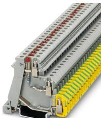
Initiator/actuator terminal block, nom. voltage: 24 V, nominal current: 24 A, connection method: Screw connection, Rated cross section: 2.5 mm<sup>2</sup>, cross section: 0.2 mm<sup>2</sup> - 4 mm<sup>2</sup>, mounting type: NS 35/7,5, NS 35/15, color: gray
