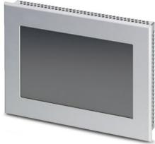
Touch panel, 17.8 cm / 7"-TFT display (analog resistive (polyester)), 800 x 480 pixel(s) (WVGA), 262144 colors, Arm® Cortex®-A8, 800 MHz, 2x USB Host 2.0, 1 x Ethernet (10/100 Mbps), RJ45, Windows® Embedded Compact 7, Movicon™, without bus system.
