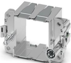
Module carrier frame, size: B06, type : for the sleeve side (A, B, C, ...), Push-in connection, 0.5 mm<sup>2</sup> ... 6 mm<sup>2</sup>, application: Module carrier frame
