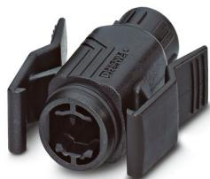
RJ45 sleeve housing, design: RJ45, degree of protection: IP67, number of positions: 8, material: PA, cable outlet: straight, color: jet black RAL 9005, Ethernet
