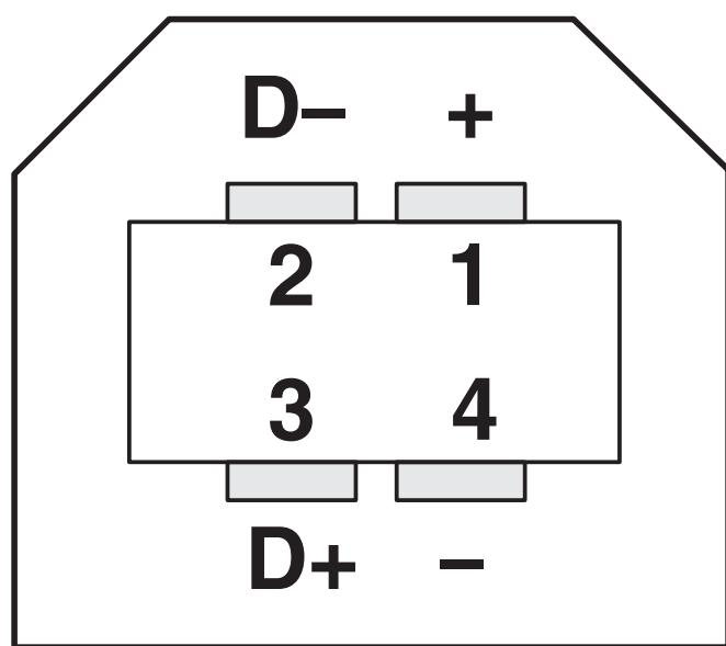
Plug pin assignment plug USB, type B
