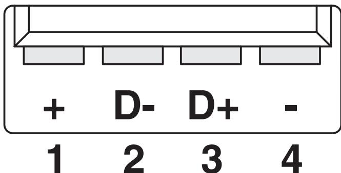
Pin assignment plug USB, type A
