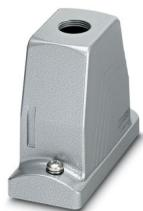
HEAVYCON ADVANCE STA sleeve housing B24, with screw locking, height 100 mm, with 2x M25 thread, straight cable outlet, with M6 x 18 hexagonal socket-head screws made of high-grade steel in acc. with DIN EN ISO 4762
