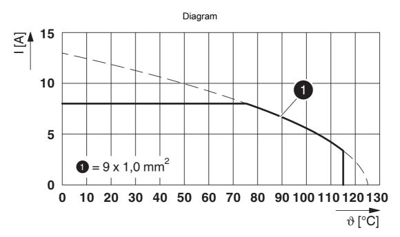
I = current strength,  $\vartheta$  = ambient temperature, 9x 8 A
