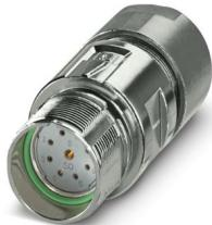
M23, Coupler connector, series: M23 PRO, straight, shielded: yes, for standard and ONECLICK fast locking system, No. of pos.: 8+1, Direction of rotation: Standard, contact connection type: Socket, Crimp connection, cable diameter range: 9 mm ... 15 mm, coding: N, Item is lead-free in accordance with RoHS II without Exemption 6c (Pb < 0.1 %)
