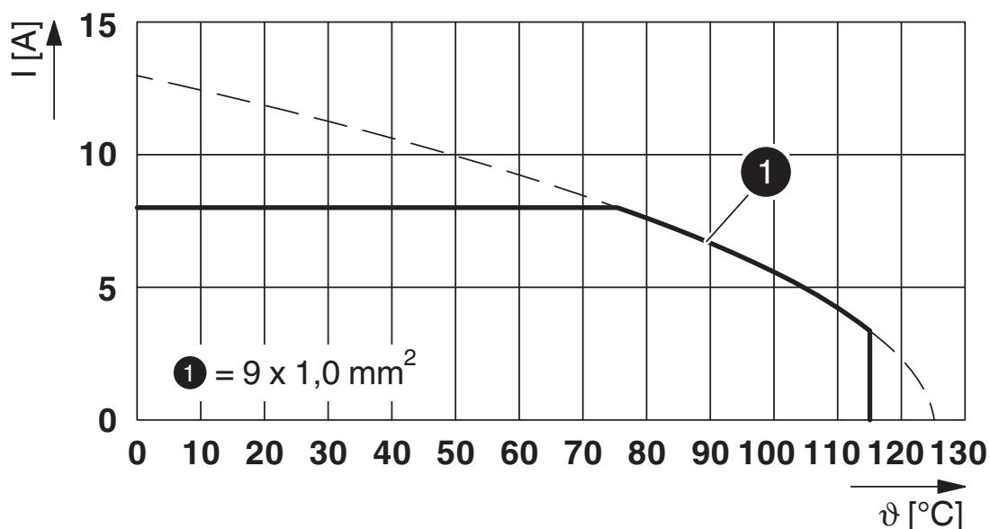
$I$  = current strength,  $\vartheta$  = ambient temperature, 9x 8 A
