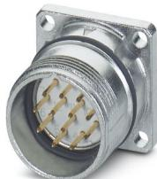
M23, Device connector front mounting, series: RC, straight, shielded: yes, Screw locking mechanism, No. of pos.: 12, Direction of rotation: Counter direction, contact connection type: Pin, Crimp connection, Axial O-ring, coding: N
