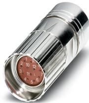
Cable connector, straight, Screw locking mechanism, M23, number of positions: 16, contact connection type: Socket, shielded: yes, cable diameter range: 9 mm ... 13.2 mm, number of positions: 16, connection method: Crimp connection, series: RF
