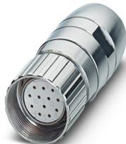
M23, Cable connector, series: UC, straight, shielded: yes, Screw locking mechanism, No. of pos.: 16+3, Direction of rotation: Standard, contact connection type: Socket, Solder cup, cable diameter range: 11.5 mm ... 13.5 mm, coding: N
