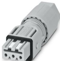
Connector, connection method: IDC connection, number of positions: 3+PE, 0.5 mm<sup>2</sup> ... 1.5 mm<sup>2</sup>, 400 V, 16 A AC/DC, gray, with one QUICKON nut, external cable diameter: 7 mm ... 13 mm, Connectors for the motor connection of Venetian blinds, blinds, roller shutters, and awnings
