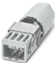
Connector, connection method: IDC connection, number of positions: 3+PE, 0.5 mm<sup>2</sup> ... 1.5 mm<sup>2</sup>, 400 V, 16 A AC/DC, gray, with one QUICKON nut, external cable diameter: 7 mm ... 13 mm, Connectors for the motor connection of Venetian blinds, blinds, roller shutters, and awnings
