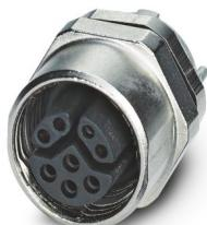
Device connector rear mounting, Ethernet CAT5 (IEC 11801:2002), 8-position, Socket, straight, M12-SPEEDCON, Y-coding, THR solder connection, this item is expected to be lead-free from Q2 2026 in accordance with RoHS II without exception 6c (Pb < 0.1%), a lead-free alternative is possible on request in advance
