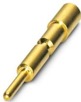
Crimp contact, Range of articles: VARIOCON, min. conductor cross-section: 0.5 mm<sup>2</sup>, max. conductor cross-section: 1.5 mm<sup>2</sup>, Connection method: Crimp connection
