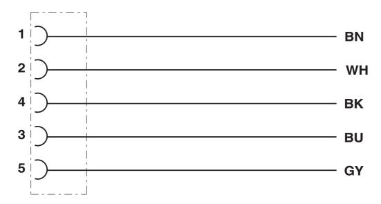
Contact assignment of the M12 socket
