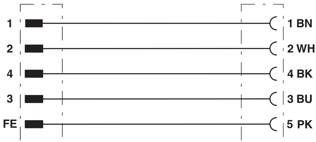
Contact assignment of M12 connector/socket
