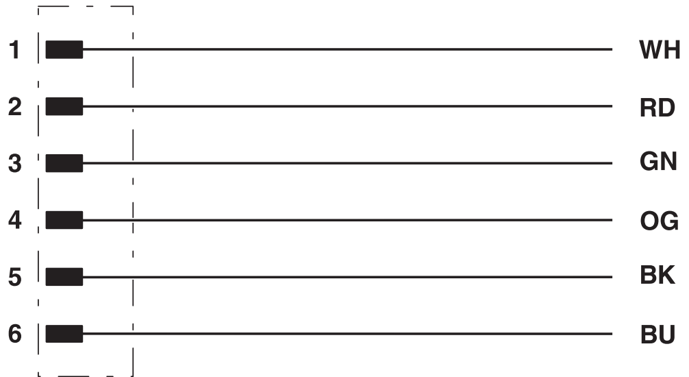
Contact assignment of 7/8" plug
