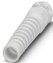
Cable gland, material for screw connection: PA, application: Standard, external cable diameter 6 mm ... 13 mm, shielding: no, connecting thread: M20 x 1.5, color: lightgray RAL 7035, with bend protection sleeve
