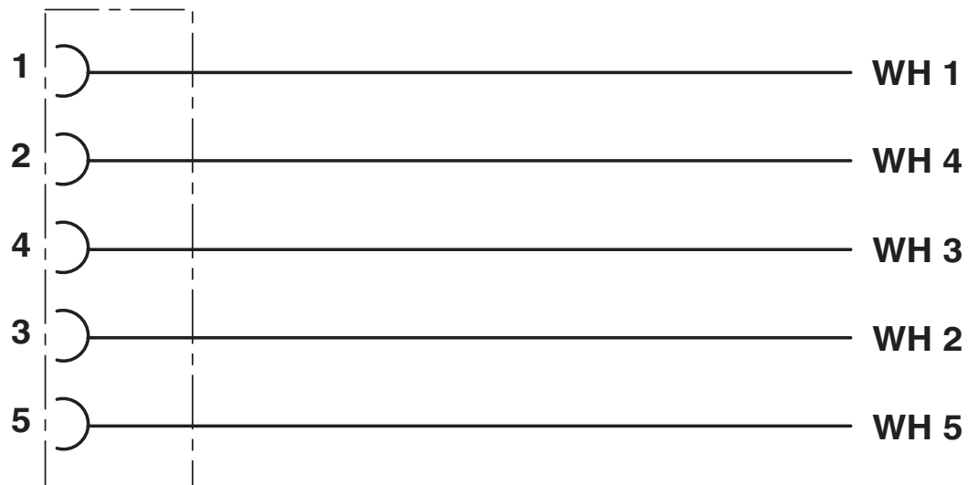
Contact assignment of the M12 socket
