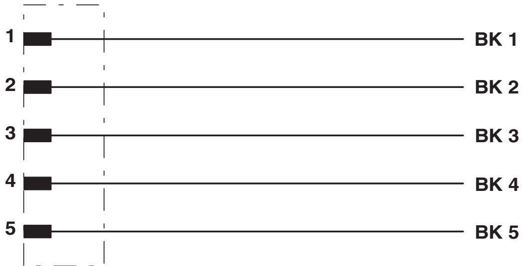
Contact assignment of the M12 socket
