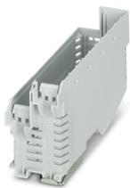
DIN rail housing, Lower housing part with metal foot catch, with vents, width: 37.89 mm, height: 120.6 mm, depth: 64.3 mm, color: light gray (similar RAL 7035), cross connection: DIN rail bus connector (optional), number of positions cross connector: 5 or 8
