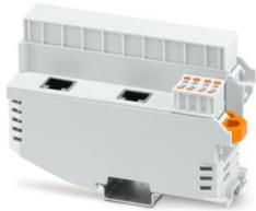
DIN rail housing, with front connection for DIN rail mounting, color: light gray (similar RAL 7035), width: 37.89 mm, height: 124.3 mm, depth: 76.5 mm, incl. 2 front connection terminal blocks, 4-pos., Push-in, for 2.5 mm<sup>2</sup>, nominal current: 8 A, 300 V, 2 RJ45 jacks, PCB surface: 10300 mm<sup>2</sup>
