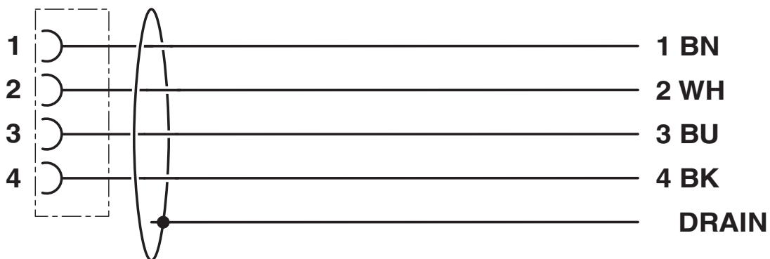
Contact assignment of M8 plugs/sockets
