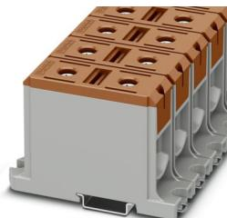
High-current terminal block, nom. voltage: 1000 V, nominal current: 290 A, number of connections: 2, number of positions: 1, connection method: Screw connection, Rated cross section: 150 mm<sup>2</sup>, cross section: 35 mm<sup>2</sup> - 150 mm<sup>2</sup>, Rated cross section: 150 mm<sup>2</sup>, cross section: 35 mm<sup>2</sup> - 150 mm<sup>2</sup>, mounting type: NS 35/15, NS 35/7,5, color: brown
