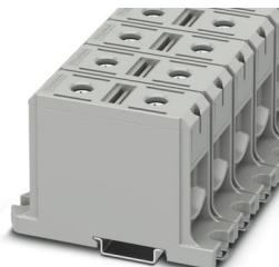
High-current terminal block, nom. voltage: 1000 V, nominal current: 290 A, number of connections: 2, number of positions: 1, connection method: Screw connection, Rated cross section: 150 mm<sup>2</sup>, cross section: 35 mm<sup>2</sup> - 150 mm<sup>2</sup>, Rated cross section: 150 mm<sup>2</sup>, cross section: 35 mm<sup>2</sup> - 150 mm<sup>2</sup>, mounting type: NS 35/15, NS 35/7,5, color: gray
