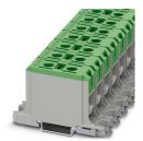
High-current terminal block, nom. voltage: 1000 V, nominal current: 145 A, number of connections: 2, number of positions: 1, connection method: Screw connection, Rated cross section: 50 mm<sup>2</sup>, cross section: 6 mm<sup>2</sup> - 50 mm<sup>2</sup>, Rated cross section: 50 mm<sup>2</sup>, cross section: 4 mm<sup>2</sup> - 50 mm<sup>2</sup>, mounting type: NS 35/15, NS 35/7,5, color: green
