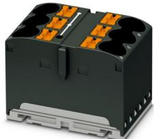
Distribution block, bridged internally, nom. voltage: 450 V, nominal current: 57 A, number of connections: 6, connection method: Push-in connection, Rated cross section: 10 mm<sup>2</sup>, cross section: 0.5 mm<sup>2</sup> - 16 mm<sup>2</sup>, mounting type: for snapping onto a DIN rail adapter, Direct mounting with flange, Free-hanging, color: black
