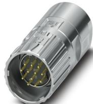
M23, Cable connector, series: M23 PRO, straight, shielded: yes, ONECLICK fast locking system, No. of pos.: 12, Direction of rotation: Counter direction, contact connection type: Pin, Crimp connection, cable diameter range: 4 mm ... 8.5 mm, coding: N, Item is lead-free in accordance with RoHS II without Exemption 6c (Pb < 0.1 %)
