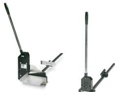
Set, comprising PPS CD M cable duct cutter, for burr-free cutting of wiring channels and their covers, can be used up to a width of 125 mm. PPS BASIC I/M rail cutter, for cutting standard DIN rails to length, NS 15/NS 35/7,5/NS 35/15 and for cutting the NLS-CU 3/10 neutral busbar to length, with inch/metric measuring rail
