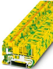
Protective conductor terminal block, number of connections: 2, connection method: Push-in / plug connection, cross section: 0.2 mm<sup>2</sup> - 6 mm<sup>2</sup>, mounting type: NS 35/7,5, NS 35/15, color: green-yellow
